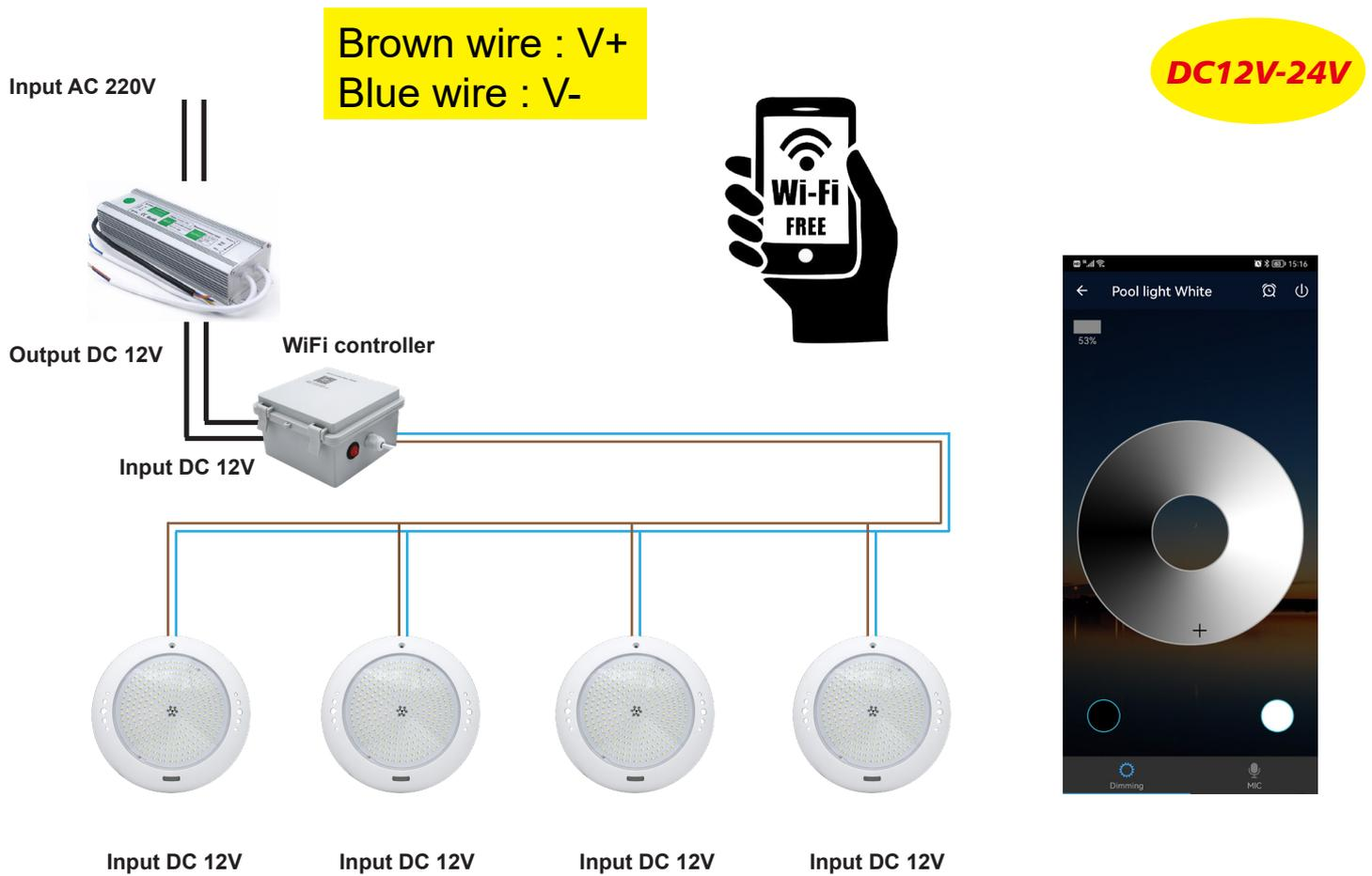
The White lights which connected with the Wifi CB004 box must be 2 wires, DC12V
